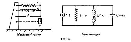
constant current generator paralleled by a resistance, inductance and capacity, and our analogous problem is to find the e.m.f. across the condenser C.
