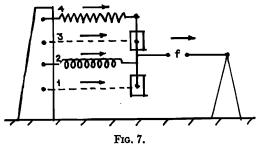
We follow the usual convention in defining mechanical impedance as the complex quotient of the force through and the velocity difference across an element or combination of elements.
